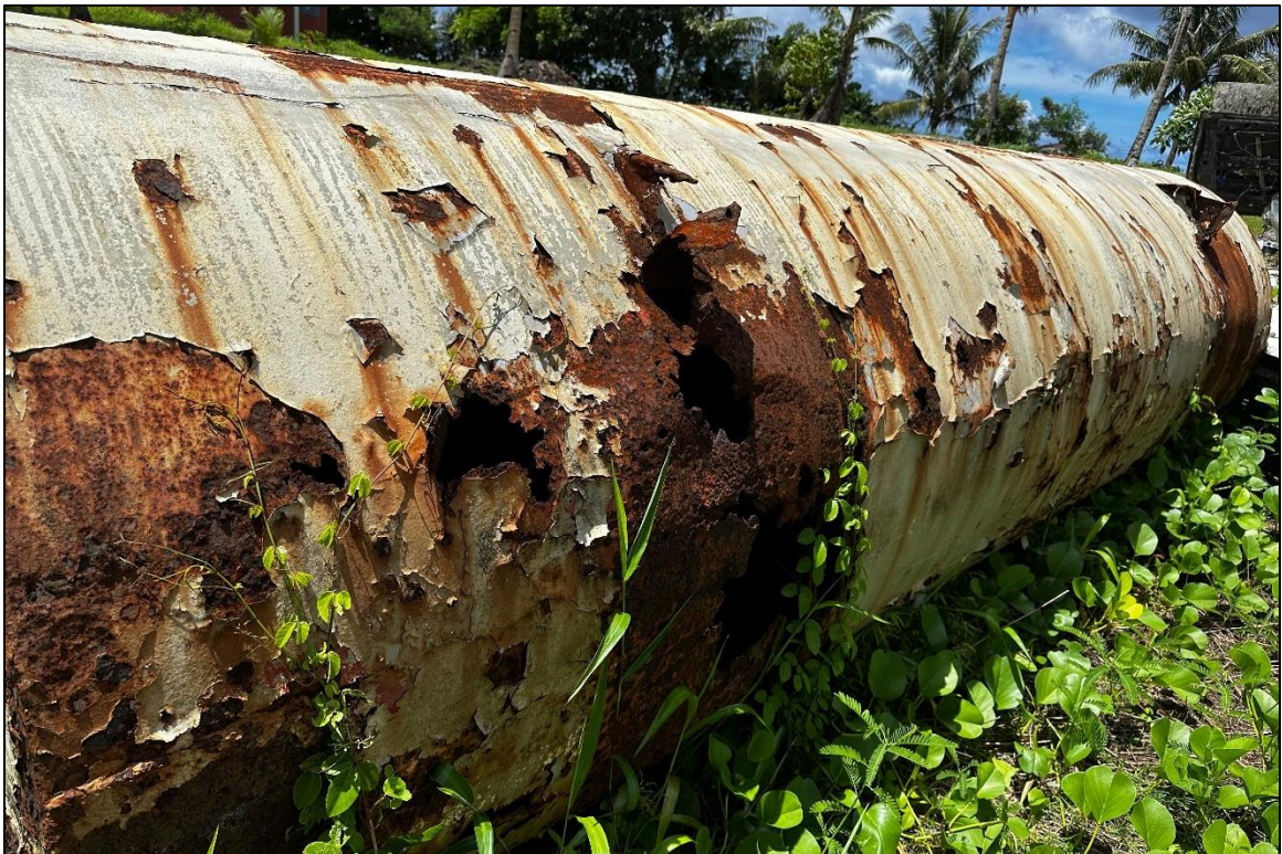
Photo 22: Close-up view of empty, deteriorated AST observed adjacent to the abandoned vehicle piles. Photo is looking west.
