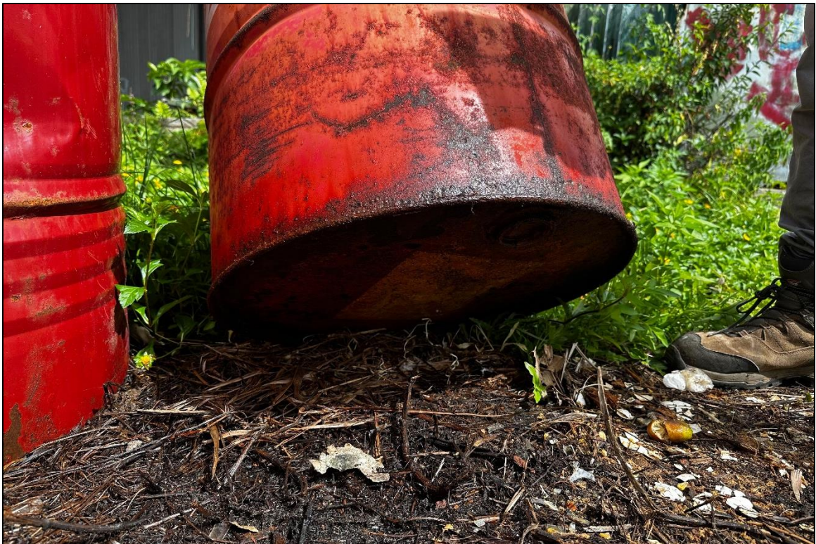
Photo 4: Close-up view of one of the four drums suspected to have leaked oily contents. Distinct petroleum odor noted emanating from dark and moist soil.
