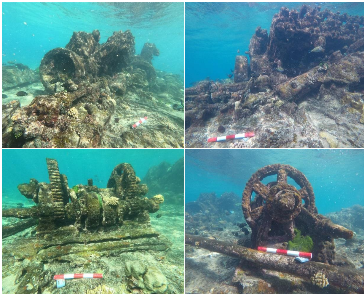
Figure 3-56 Propulsion Engine (Top Left and Top Right) and Windlass (Bottom Left and Bottom Right) (Photos by AECOM)
