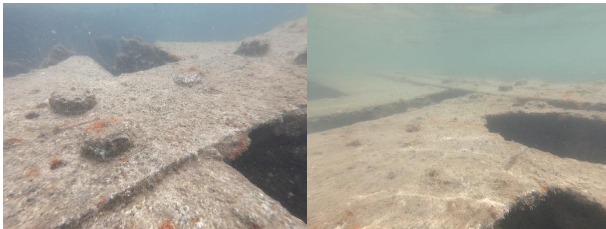
Figure 3-116 Single Riveting Butt Straps and Deck Plating (Photos by AECOM)
