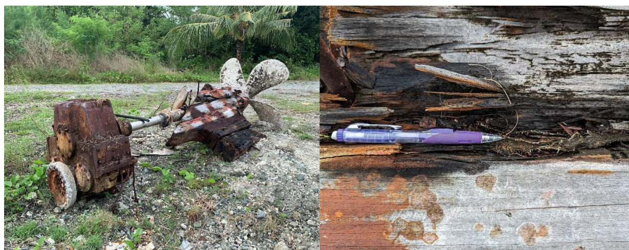
Figure 3-79 Engine, Propeller, Prop and Shaft, and Fiber Insulation on Target 04 (Photos by AECOM)
