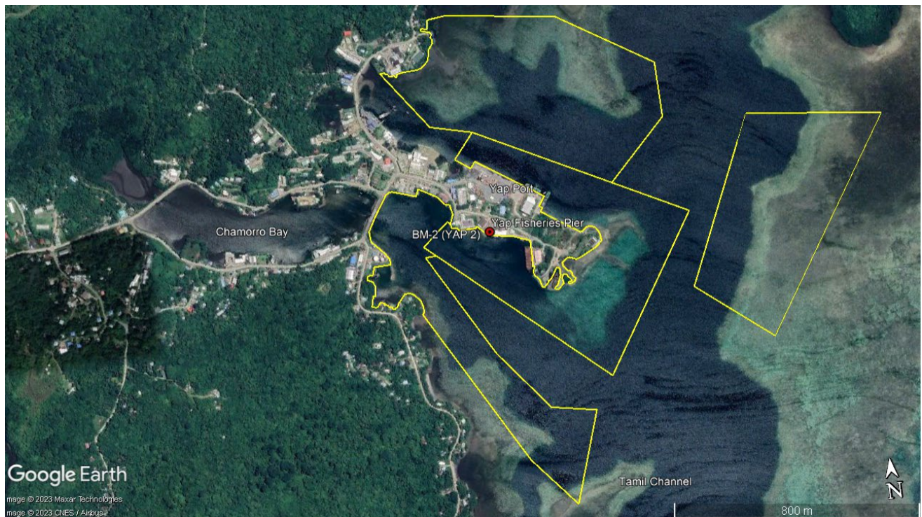
Figure 2-1. Benchmark BM-2 (YAP 2) location marked in red, with respect to the harbor survey areas outlined in yellow
