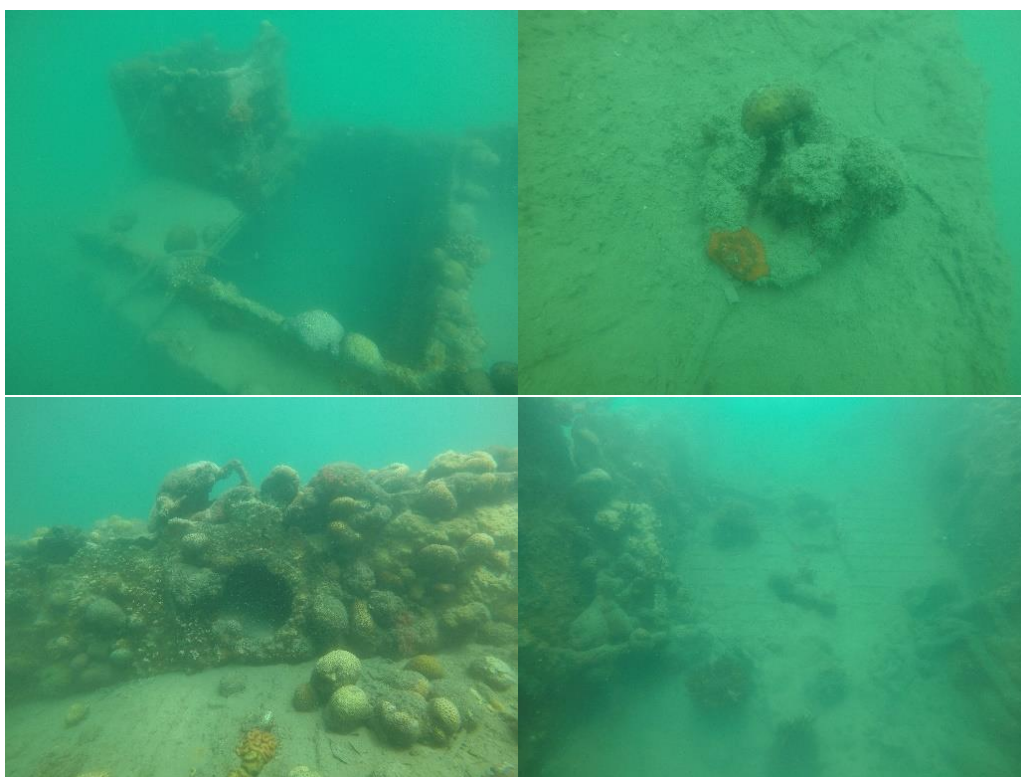
Figure 3-108 Pilot House (Top Left), Cargo Tie Rings (Top Right), Access Holes to Wing Tanks (Bottom Left), and Corrugated Flooring (Bottom Right) on Target 16 (Photos by AECOM)
