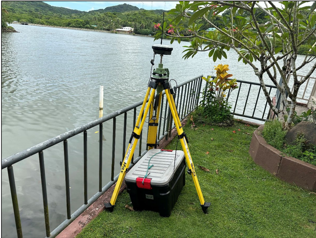
Figure 2-5. Leica GS-16 GPS base station
