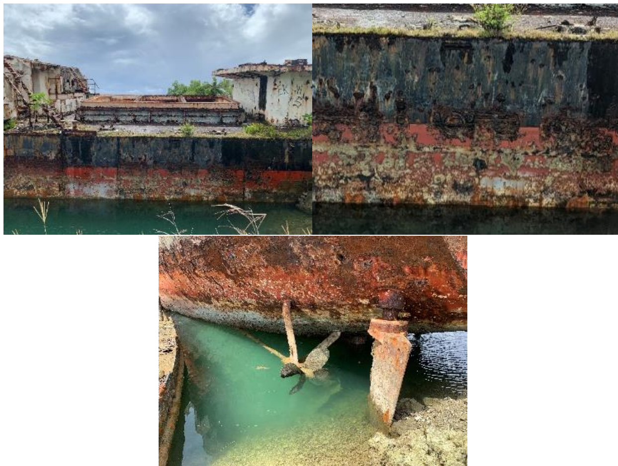
Figure 3-64 Welded Deck Plating, Plimsoll Mark, Fixed Skeg, and Rudders on Target 01 (Photo by AECOM)
